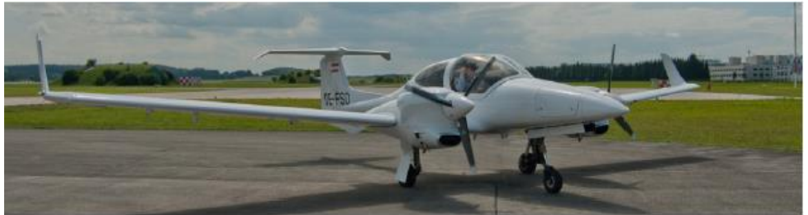
Fig. 1 Research Flying Testbed (DA-42MPP NG) featuring EFbW FCS
